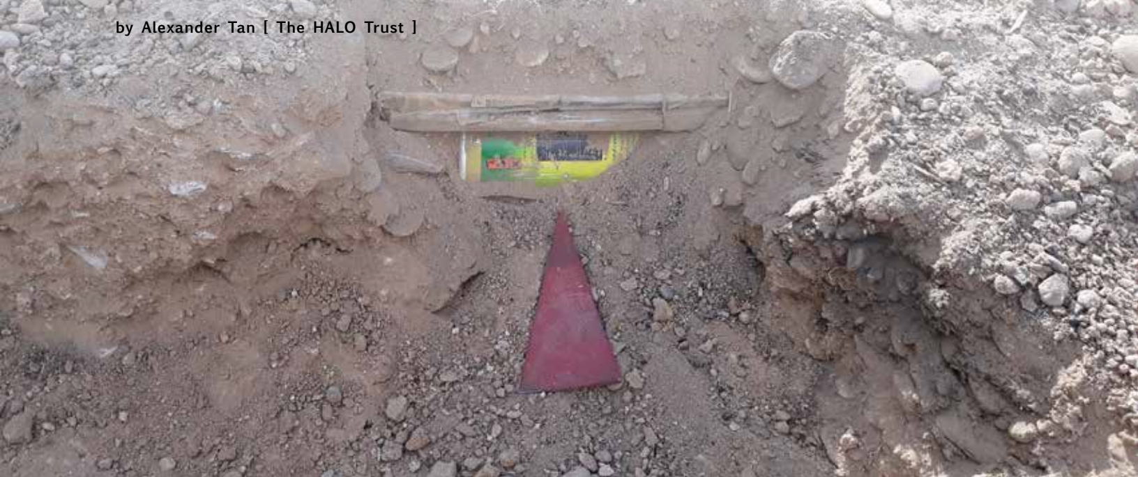
Image 1. The first abandoned improvised mine (AIM) uncovered by HALO clearance teams in Helmand Province, southern Afghanistan. All images courtesy of The HALO Trust.
