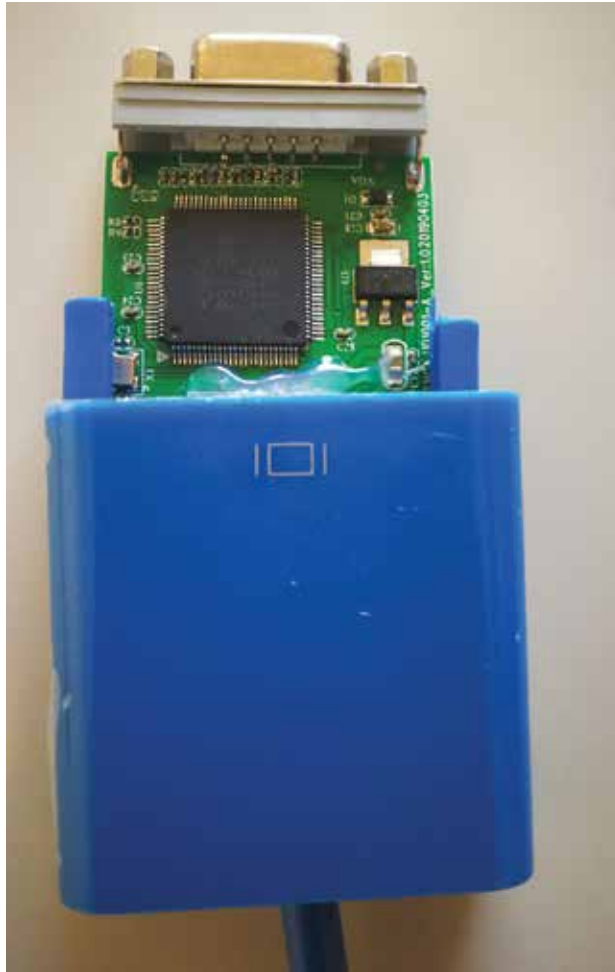
Image 1. Photo of the SDR chip inside a USB 3.0-to-VGA adapter.
