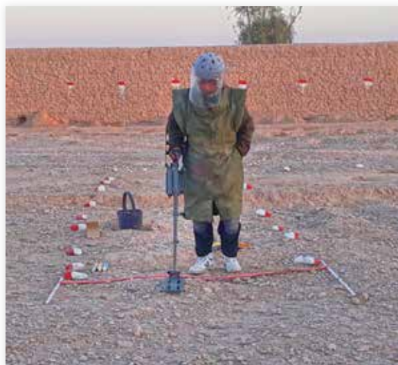
Images 6 (left) and 7 (right). An example of the standard Afghanistan “one man, one lane” (OMOL) technique with a searched area of 1.4 m x 0.3 m, compared to the HALO AIM 2 m breaching technique with a searched area of 2.4 m x 70 cm.
