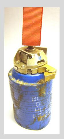
The SD is a pyrotechnic fuse which should be ignited as the bomblet arms in flight, and which burns for 15 seconds. Should the primary impact mechanism fail when the bomblet hits the target/ground, then the SD fuse should set off the detonator, normally 5-7 seconds after impact.
