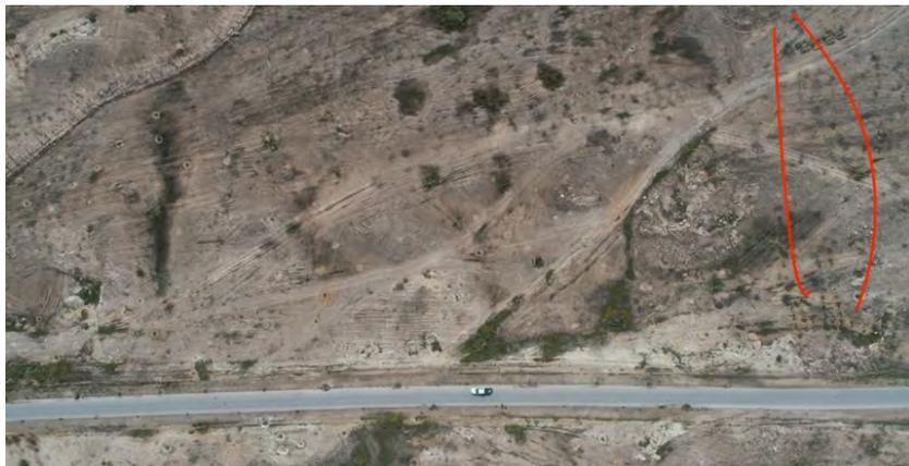
Figure 9.5 Identification of a mine row in the right part of the image. [ Mats Hektor, NPA South Iraq].
