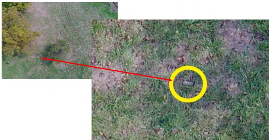
Figure 3.3 Detection of the landmine in Blagovac, in the color visible image from RPAS. [NPA Bosnia and Herzegovina]
