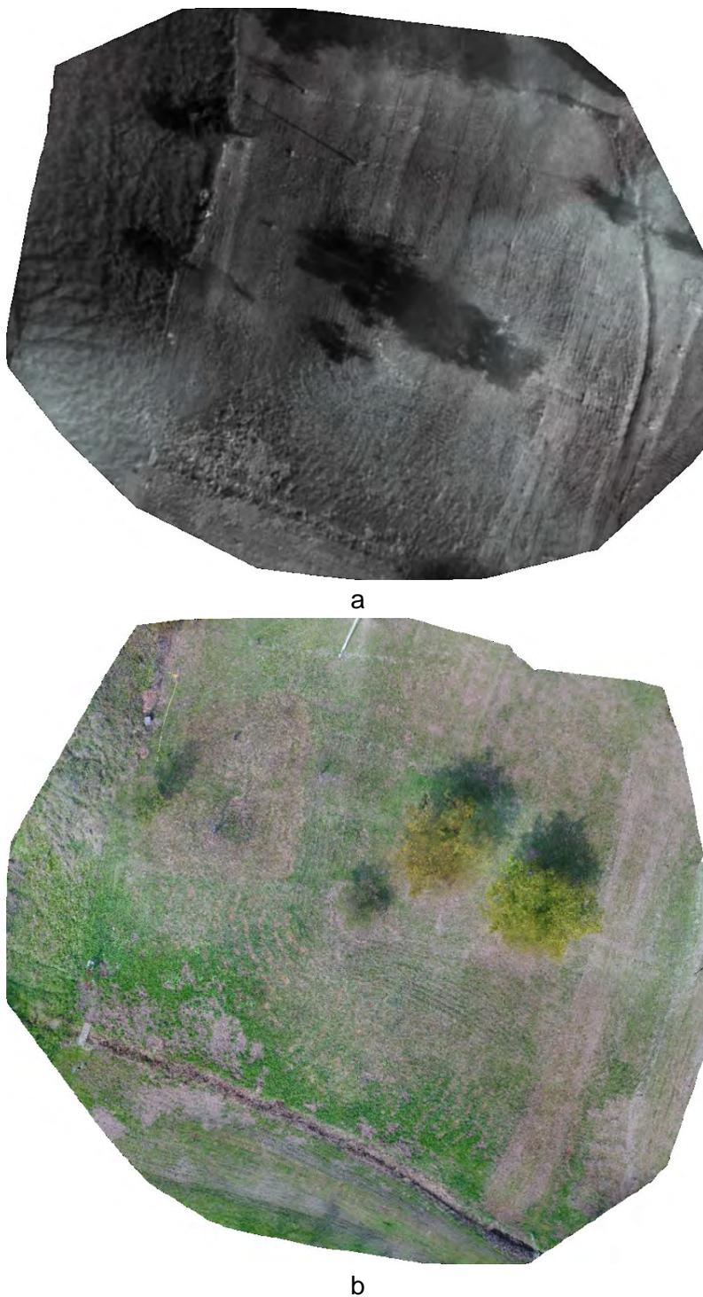
Figure 3.8 a) Thermal infrared mosaic of NPA Bosnia test site Blagovac, b) color visible mosaic derived from recordings acquired October 2019. [NPA Bosnia and Herzegovina].
