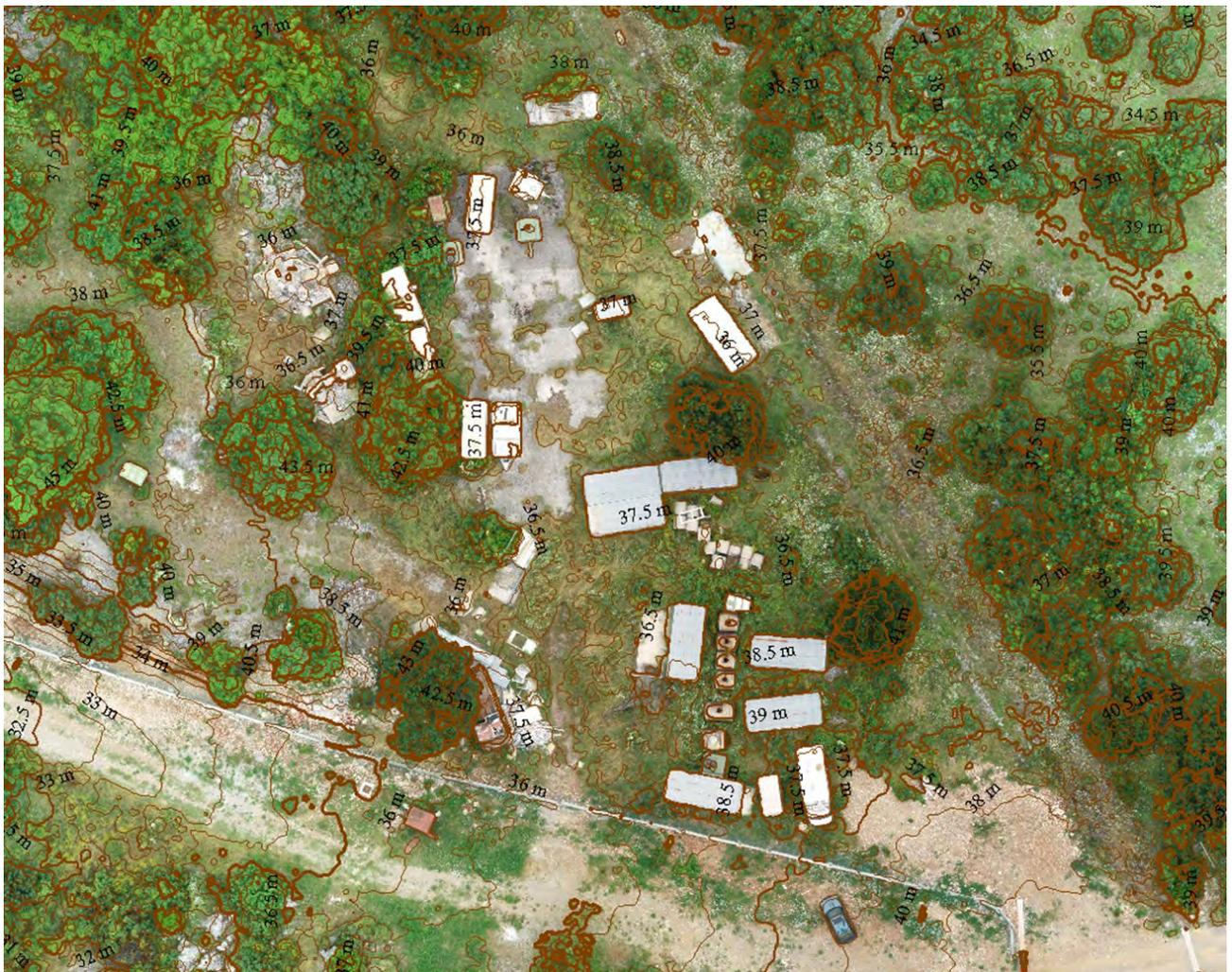
Figure 2.7 The contour lines overlapped onto the color visible mosaic.
