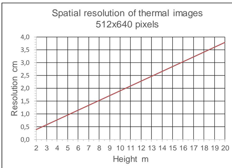
Figure 11.1 Diagram shows a relation between flight height and the spatial resolution of the thermal infrared images
