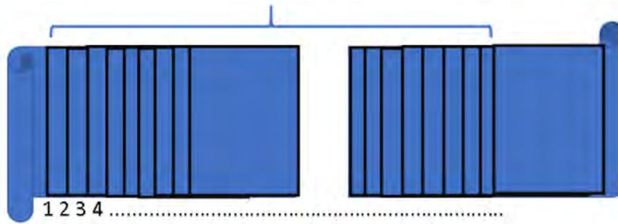
Figure 4.2 The TIR video recording can be exported into a sequence of images (frames), every frame has 720x480 pixels, with a frequency of 30 frames per second.
