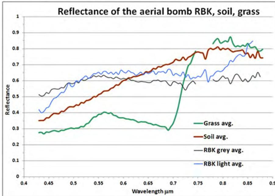
Figure 8.5 Reflectance spectra of the aerial RBK bomb, of the grass and the soil surface, [24].
