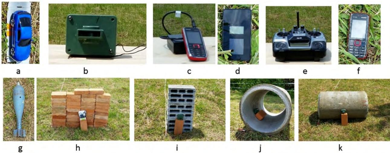
Figure 8.2 The targets detected by a manual NLJD, a – g. Targets behind or inside of the obstacles, h – k.
