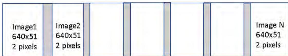
Figure 4.1 TIR images are used with overlapping, the greater overlapping the better mosaic can be produced.
