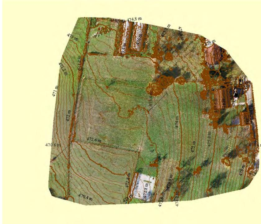
Figure 3.12 Contour lines overlaid on the color visible mosaic of Blagovac.
