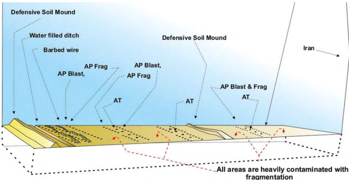
Figure 9.3 Scheme of the minefields between Iraq and Iran. The region of the Non-Technical and Technical Survey in South Iraq. Note the remnants of barbed wire on the left side of this figure and in Fig. 9.4. [ Mats Hektor, NPA South Iraq].
