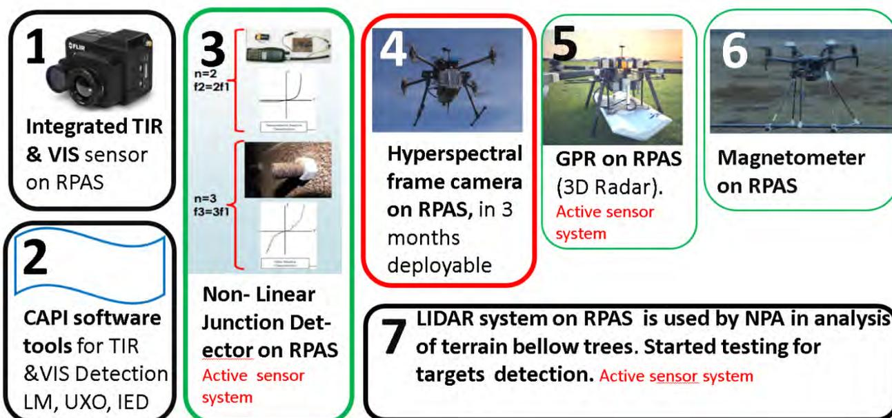
Figure 8.1 The sensors that are in use in NPA and the sensors recommended for future implementation in NPA survey technology.
