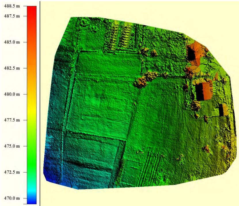
Figure 3.10 a) DSM of Blagovac derived from LIDAR recordings collected via RPAS on 30.10.2019
