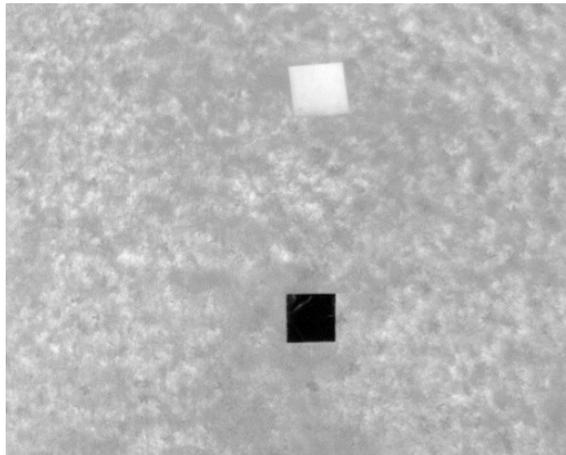
Figure 11.2 The calibrating targets in a thermal infrared image: the polished aluminum target appears black, while the black-painted cardboard plate appears white.
