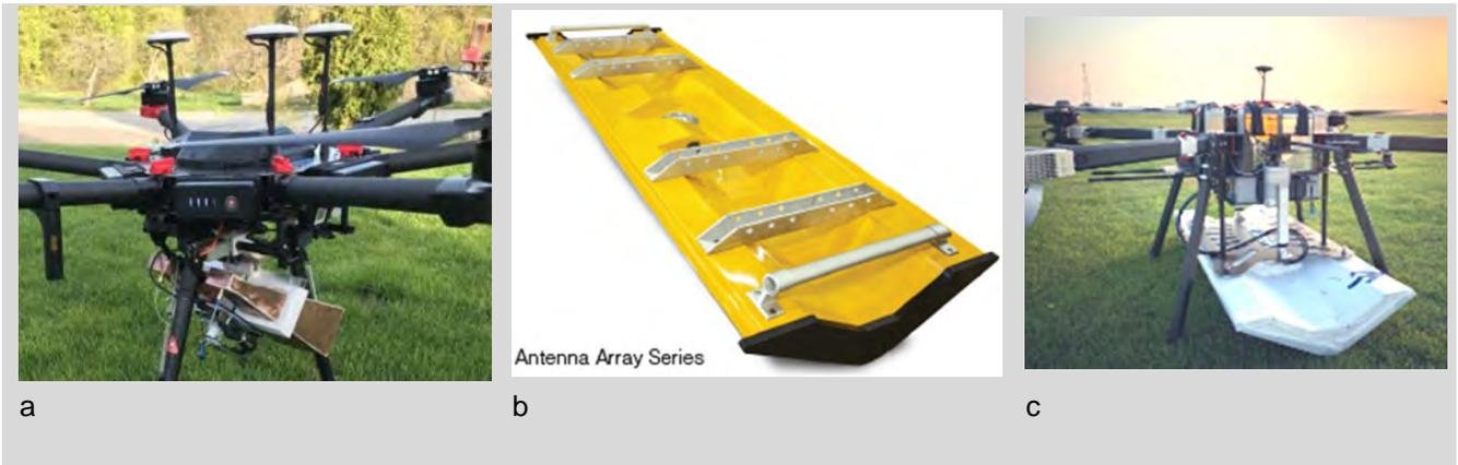
Figure 8.6 a) GPR developed at FERl, University of Maribor, Slovenia, [25]. b) Antenna a key part of GPR produced by Norwegian company (3-D RADAR), [26]. c) One concept of the GPR for use from industrial RPAS, [no-name photo on the Internet].
