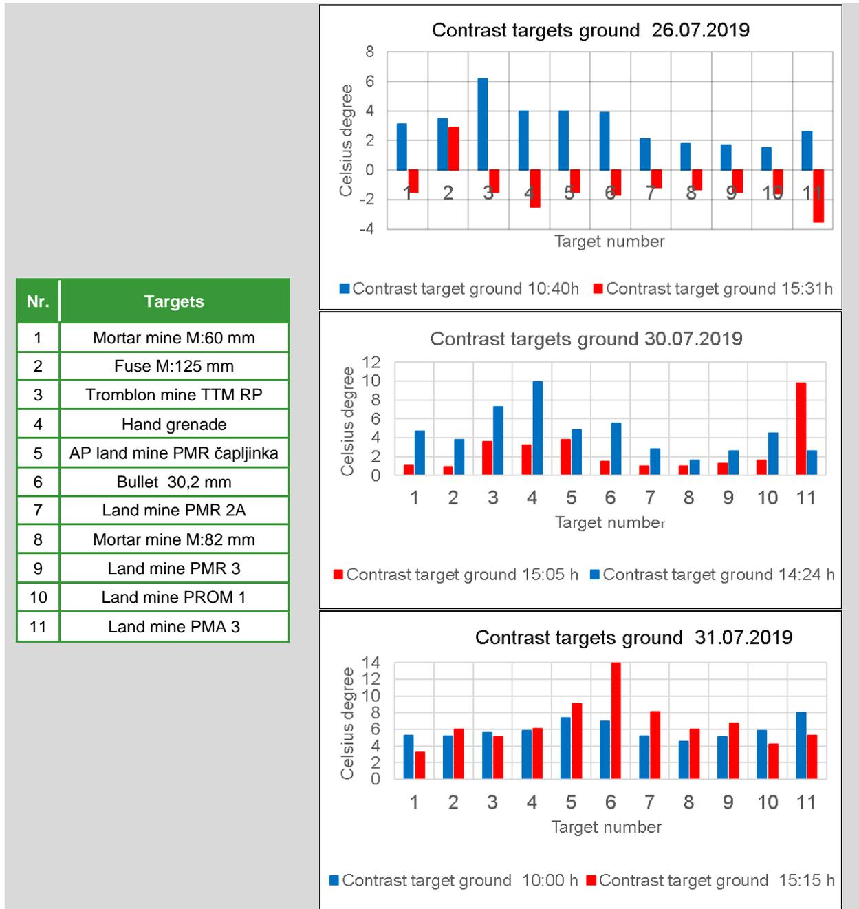
Figure 4.7 Targets used in measurements of the thermal contrast and diagrams of data for three days in Blagovac in July 2019.
