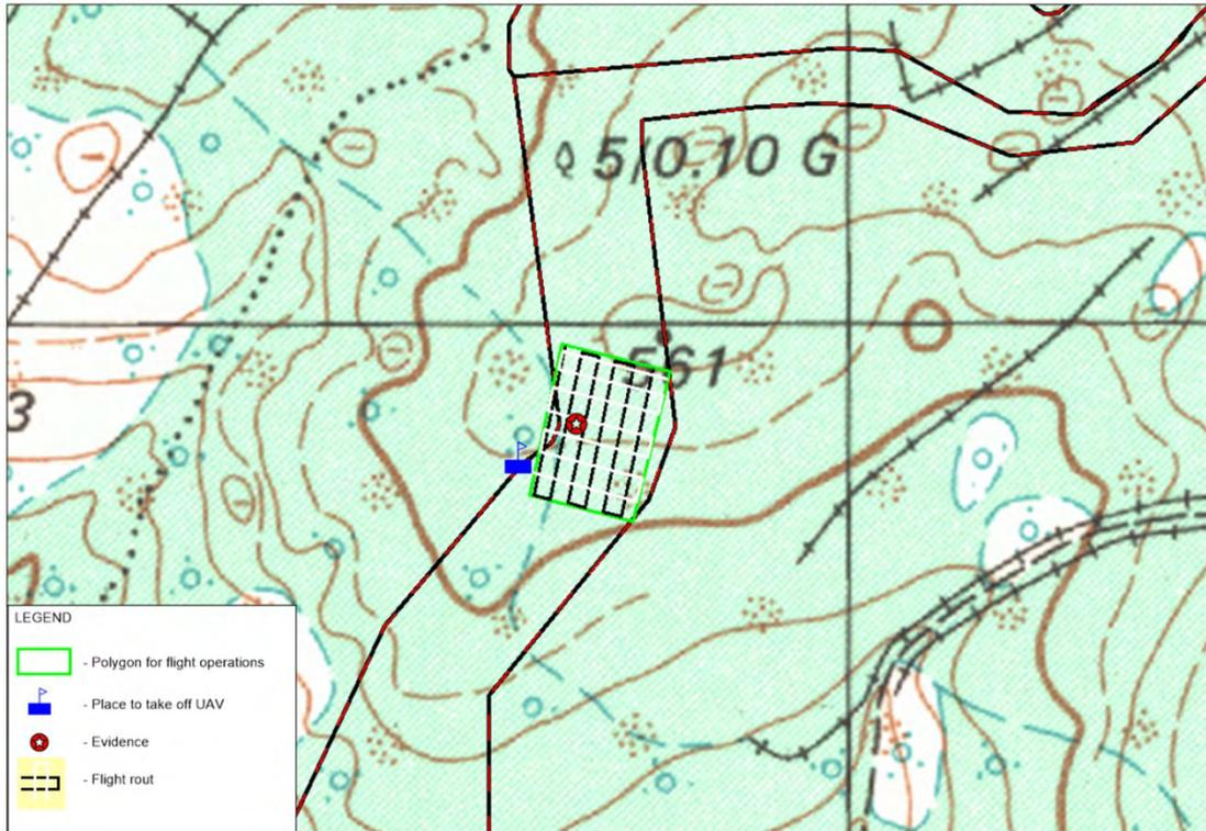
Figure 3.4 The detection of a landmine in Rotimlja, by watching the color visible images and video acquired via RPAS. [NPA Bosnia and Herzegovina]
