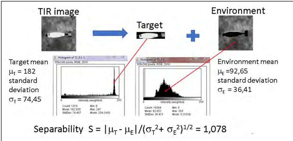
Figure 4.4 The definition of the separability and the example for the Mortar mine M 60.
