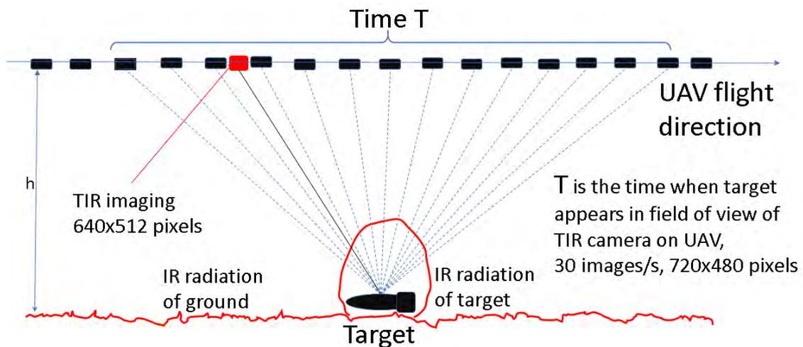
Figure 4.3 When RPAS flies at height  $h$  above the target on the ground, with speed  $v$  (m/s), the TIR sensor receives thermal infrared radiation of the target during the time  $T$ . In thermal video frames (720x480 pixels) this happens more often, see example Tab. 4.1.
