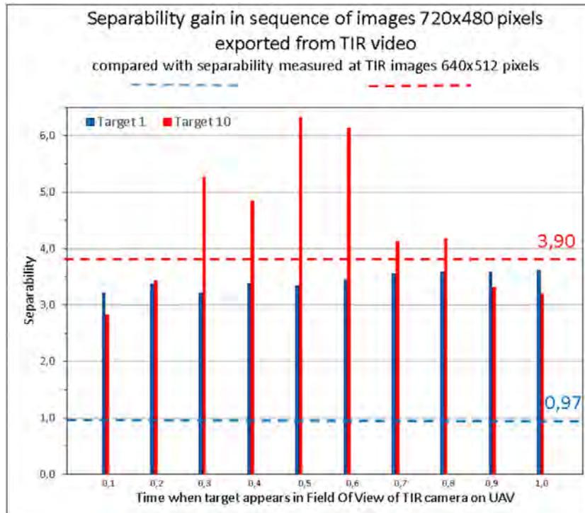
Figure 4.5 Separabilities obtained from thermal image 640x512 pixels (dashed lines) and thermal frame 720x480 pixels, vertical lines. A target 1 is a mortar mine M60 mm (blue lines), a target 10 is a land mine PROM1 (red lines).
