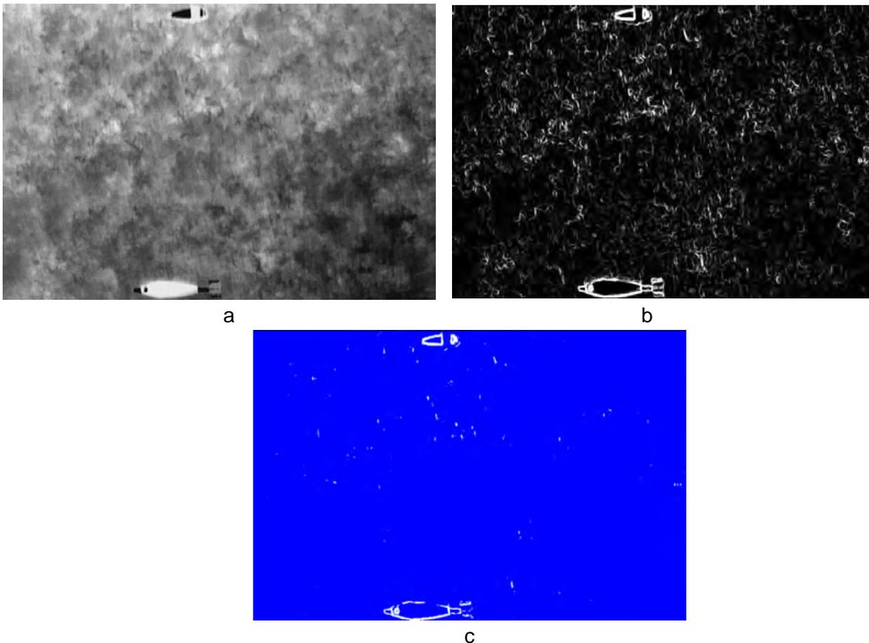
Figure 7.1 Tool for the detection edges of targets in the thermal infrared image, and in the sequence of thermal images. a) Two targets in 720x480 pixels image, b) The enhanced edges of targets, c) The clutter suppressed.
