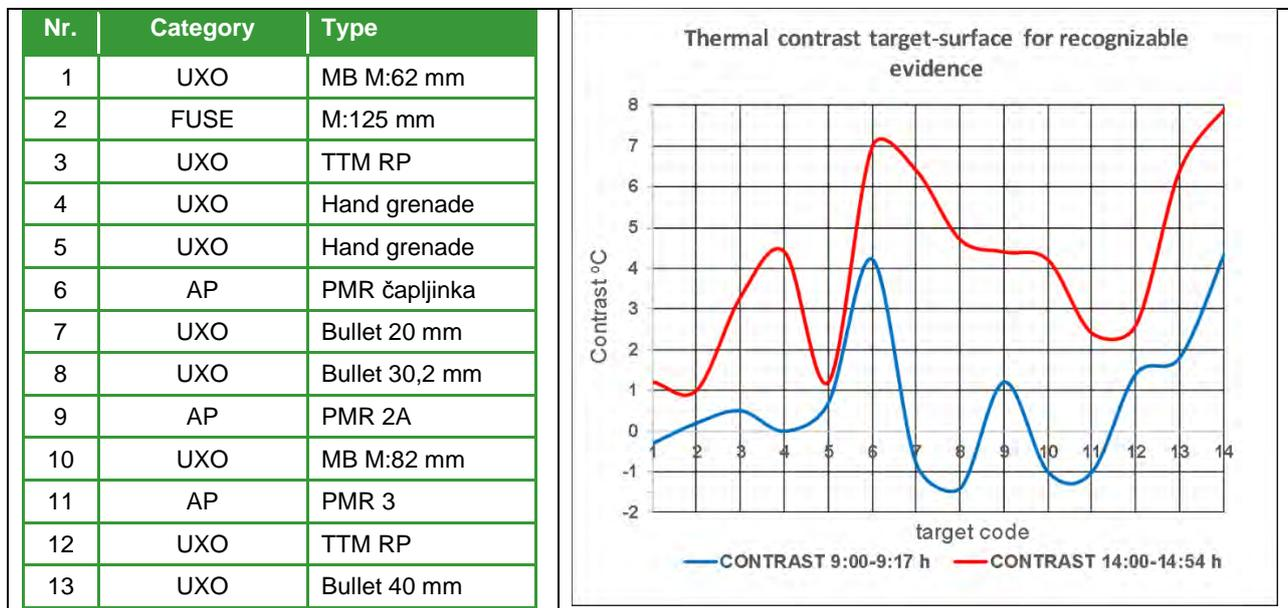
Figure 4.6 List of the targets used for testing their TIR detectability, and diagram of a measured thermal contrast between the target and the ground surface. Blagovac 2018.
