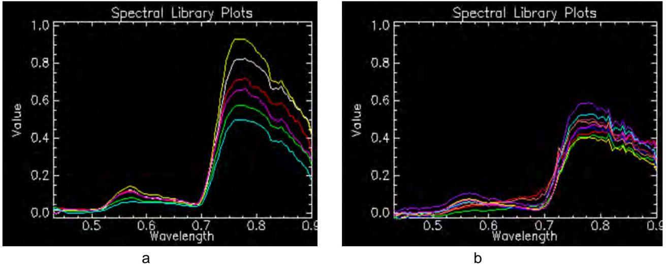
Figure 8.4 a) Spectra of the grass in the minefield, b) spectra of the grass outside of the minefield, [24]
