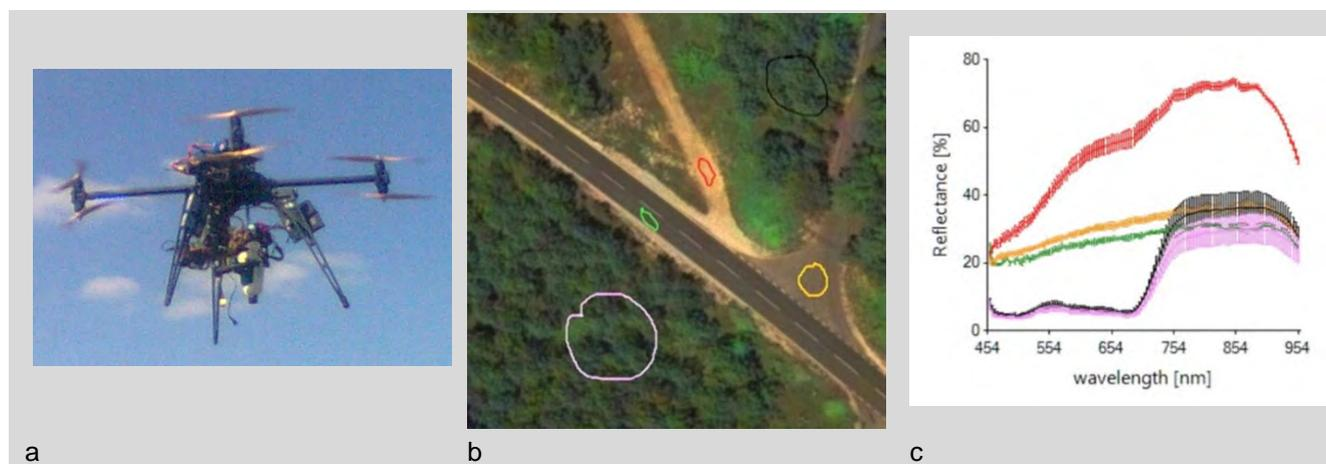
Figure 8.3 a) The hyperspectral frame camera on the RPAS. b) The example of the ground scene marked areas for the analysis of the spectra. c) Reflectance spectra of the selected areas in b), [24].
