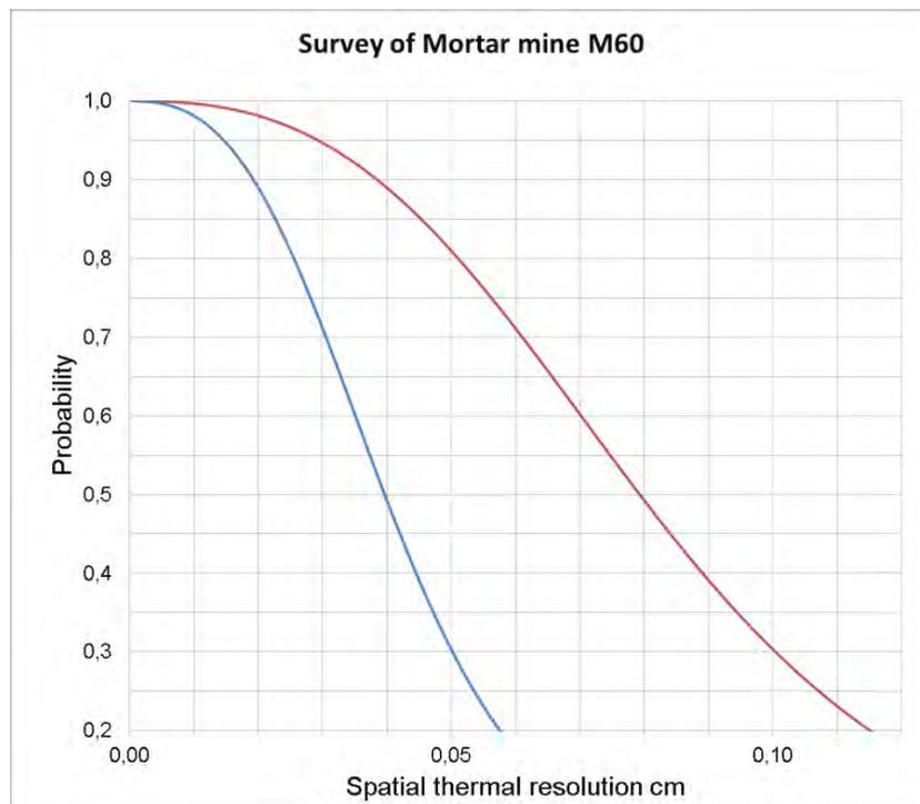
Figure 6.5 Probability > 0,2 of detection (red), classification (blue) of a mortar mine M60 in a thermal infrared image
