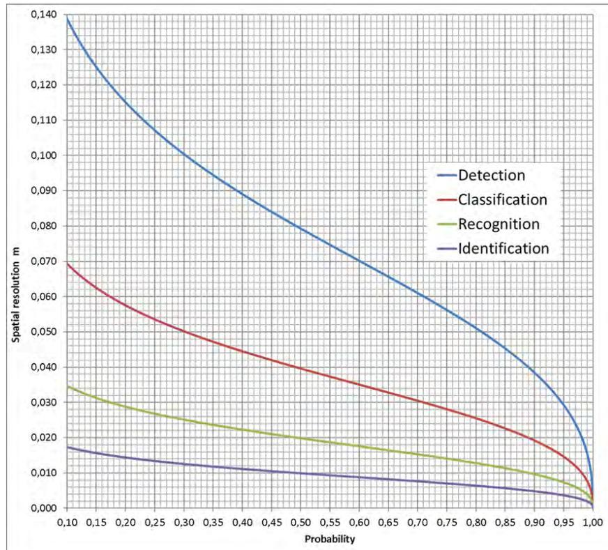
Figure 5.2 Spatial resolution of thermal infrared images needed for the selected probability of survey functionalities detection, classification, recognition, and the identification, for mortar mine
