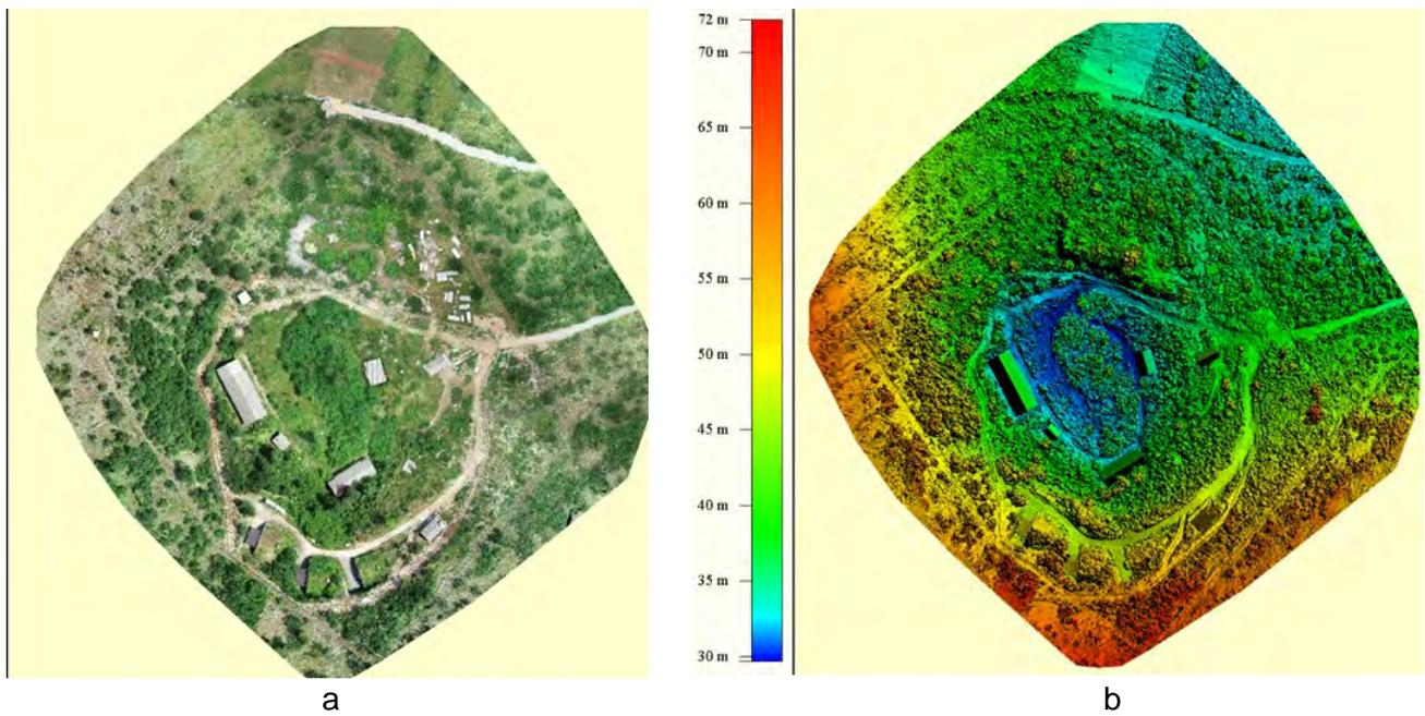
Figure 2.5 a) Color visible mosaic, b) digital surface model (DSM) of the ASA Rogami. [NPA Bosnia and Herzegovina]
