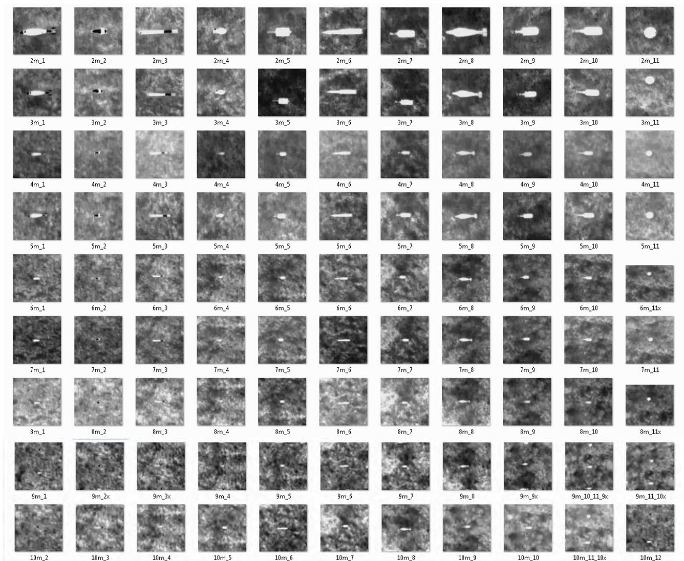
Figure 6.2 The thermal images for each target at increased flight height, from 2 m to 10 m, by step 1 m.
