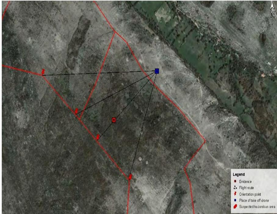
Figure 3.6 Test of the non-technical survey based on the color visible image collected via RPAS in the region Kamena. The evidence derived from this image approved the existence of the secondary indicators of the contamination, shown on the next figure, the trench, and the dry-stone wall. Image of Kamena, [NPA Bosnia and Herzegovina]
