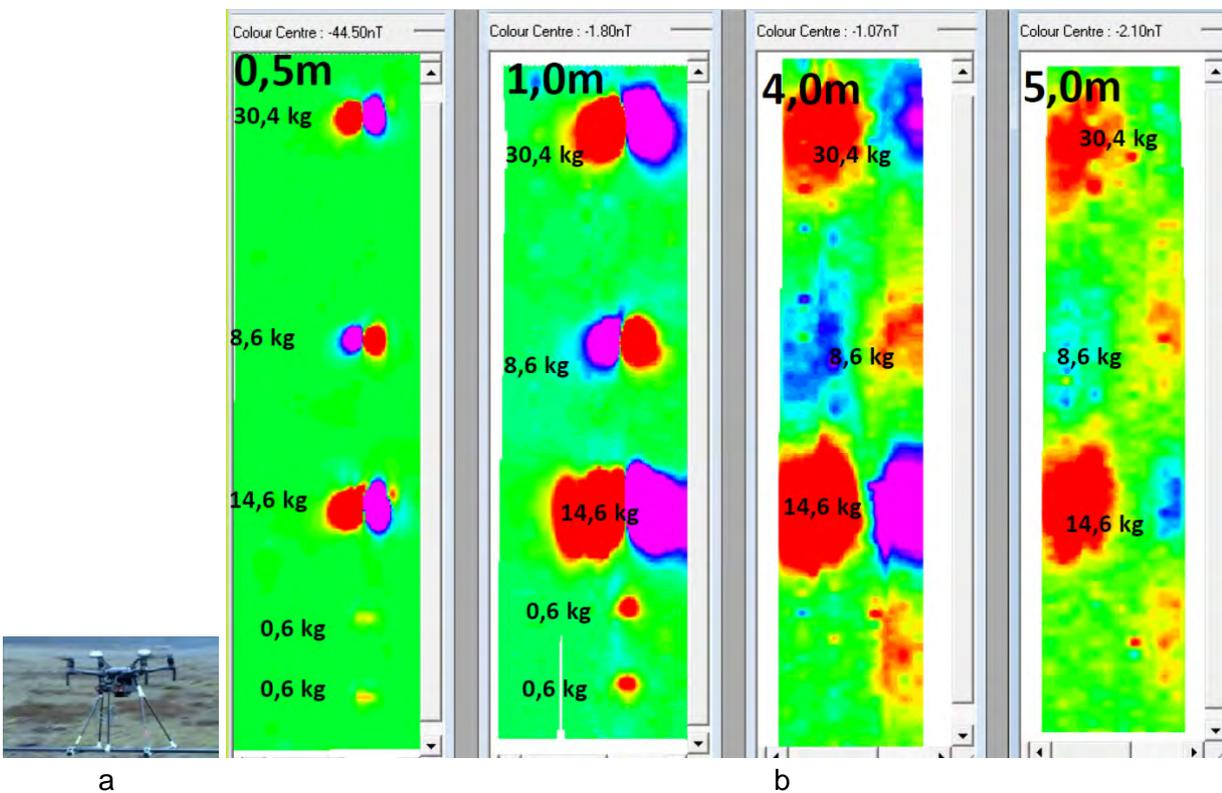
Figure 8.7 a) Magnetometer on RPAS. b) Results of testing in Allentsteig, Austria. The precision of locating UXO depends on the strengths of the magnetic field in nT (top of each sub-image), which is dependent on the mass of UXO and its distance to a magnetometer.
