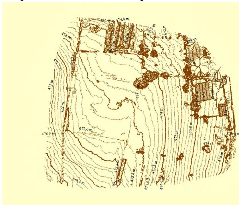
Figure 3.11 Contour lines of Blagovac derived from LIDAR data collected via RPAS on 30.10.2019.
