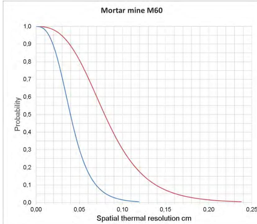
Figure 6.4 Probability of detection (red), classification (blue) of a mortar mine in a thermal infrared image
