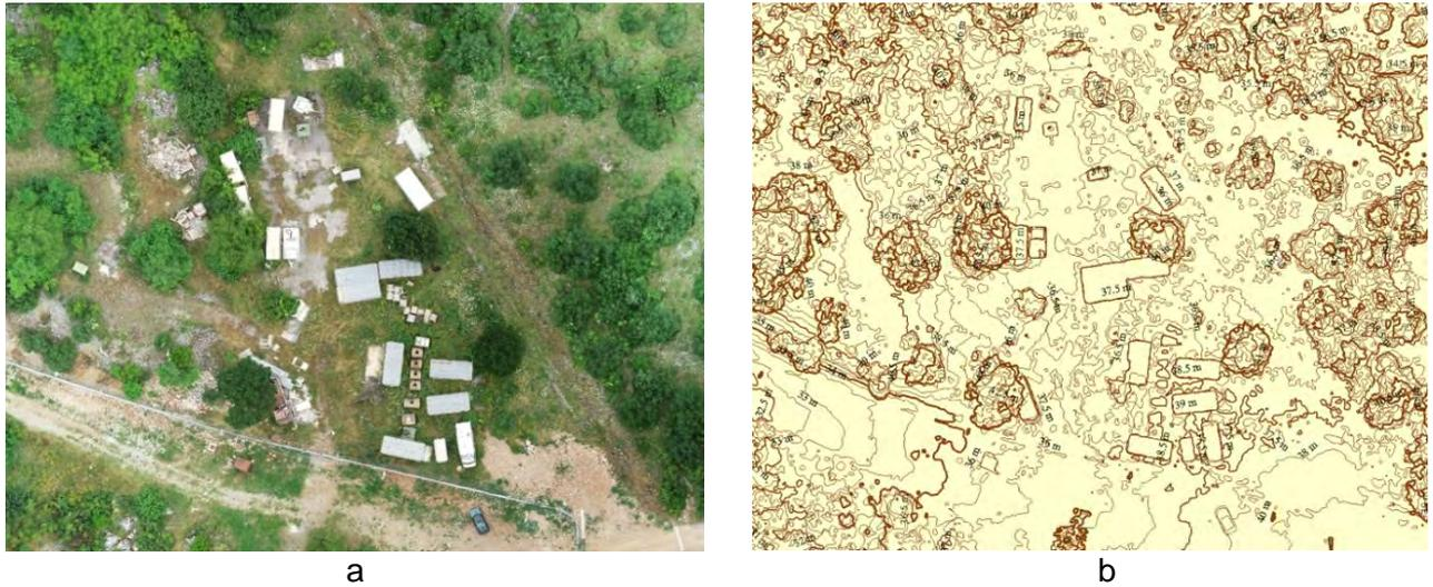
Figure 2.6 a) Part of the color visible mosaic of the eastern part of ASA Rogami, b) contour lines derived from DSM of the same area. The contour lines show the relative heights of surface objects.
