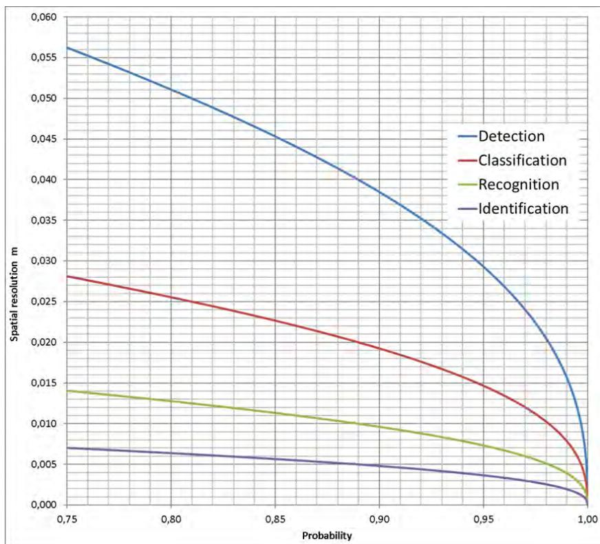
Figure 5.3 Spatial resolution of thermal infrared images needed for the selected probability of survey functionalities detection, classification, recognition, and the identification, for mortar mine, in probability range from 0,75 to 1,0.
