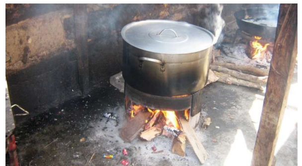
Before Photo: Traditional Inefficient cookstoves (open fire/ 3-stone fire) with increased air pollution.
