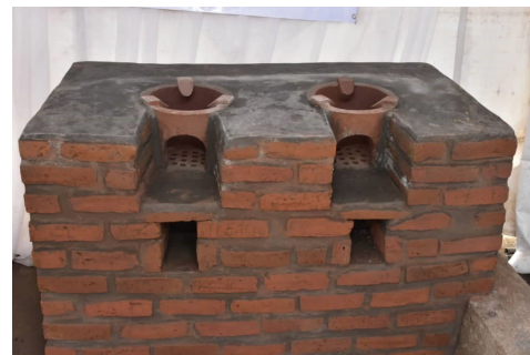
After photo: Efficient & Improved Biomass cookstoves with reduced emissions.
