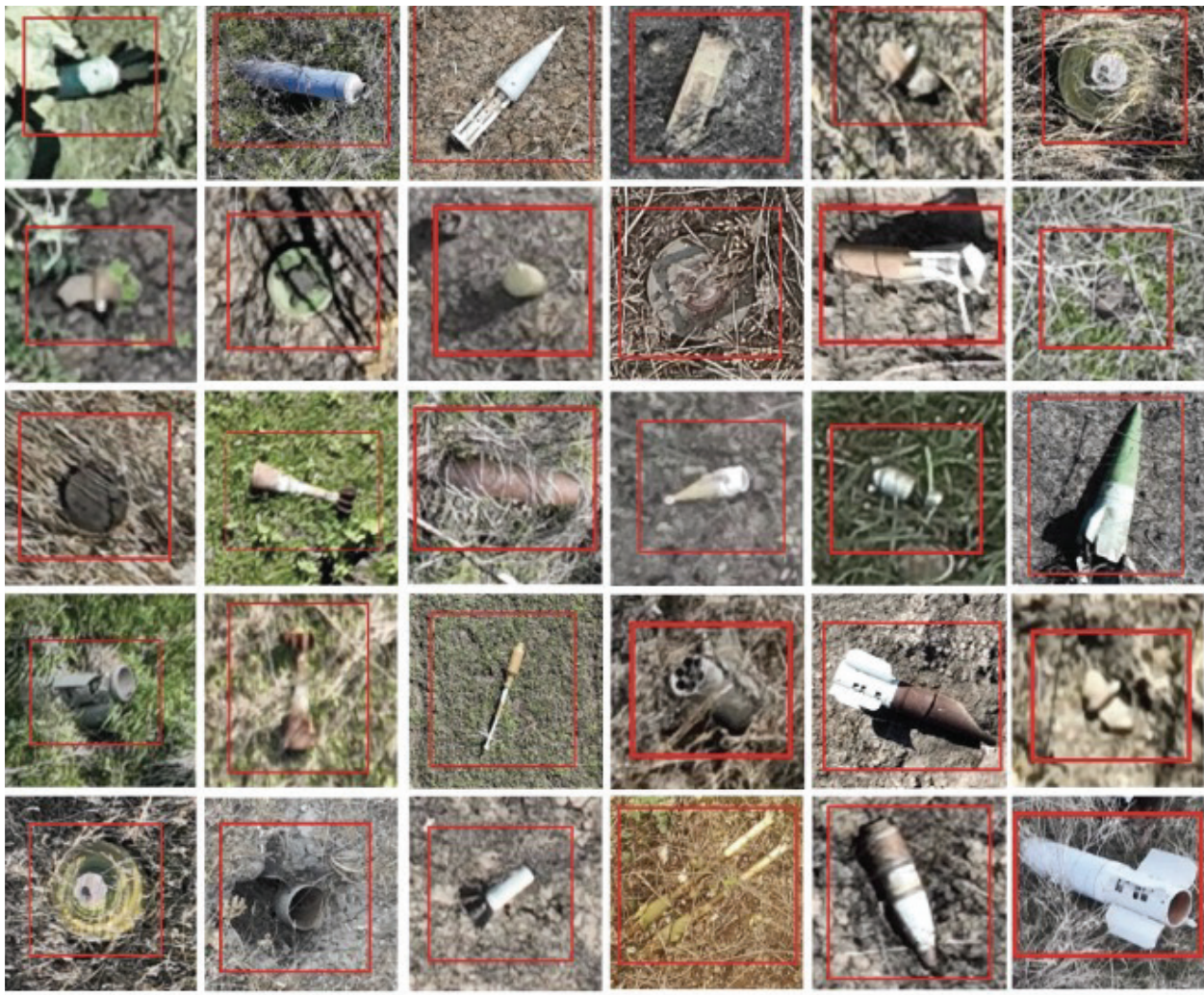
Figure 2. Examples of direct evidence points detected by SpotlightAI from drone imagery. The red box shows the machine learning model prediction. Detected items range from BM-21 Grad rockets, TM-62 anti-tank mines, various submunitions, and small anti-personnel mines. (Image courtesy of Safe Pro AI)
