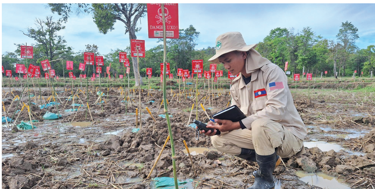
NPA Deputy Team Leader Sakda Leuamnard photographed on 15 May 2025, using a GPS device to record the coordinates of unexploded submunitions in Phornuan village, Paksong district, Saravane province, Lao PDR. Each sign indicates one identified unexploded submunition. Photo: NPA Lao PDR.
